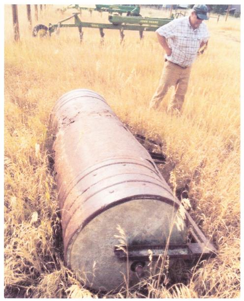
Having struggled with rocks, large brush and stumps, here is my latest contraption to try making the banks and Right-Of-Ways more mowable. I've rented a roller from one of our neighbors that is wider than the tractor and weighs well over a ton. Most places will require a couple of passes.
