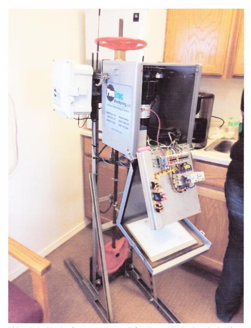
This might be the future. We are all familiar with the hand wheel seen here at the top, to open and close a take-out. The little plate at the bottom is normally hidden under the water but it is driven by the hand wheel and controls water flow past it. All that modern looking box and wiring, in the middle, will allow all control of this device from either a cell phone or automatic scheduling. How un-stimulating!!
